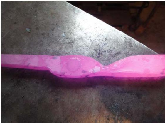
Turn the half tong over to see the "eye" on the back. Center your punch on the eye, give it a couple of good whacks, then move to your anvil's pritchel hole and drive the punch farther, knocking out the "biscuit" (the slug). Remove and quench your punch.
