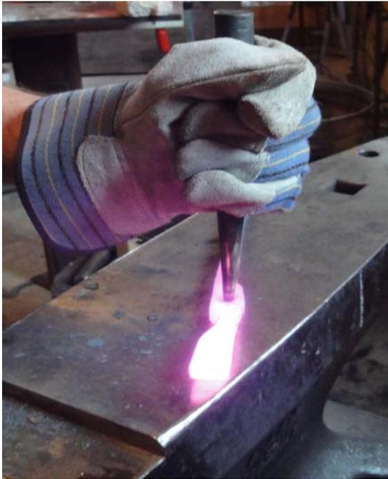
Punch holes for a rivet at the hinge. Heat the hinge area to yellow. Drive your punch down with a heavy hammer, until you can feel the punch bottom out. Quench your punch after every two blows. If you let the punch get overheated, it will mushroom.
