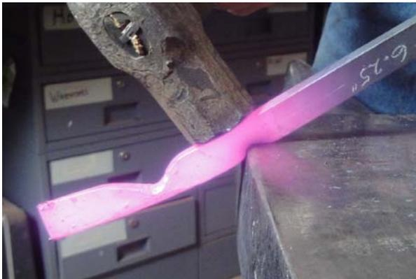
Using the rounded far edge of your anvil, forge a rounded notch in from the side of the bar at the second mark. Go a little less than halfway through the bar.
