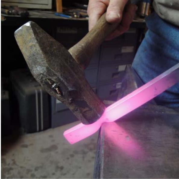
Using the rounded edge of your anvil, forge a rounded notch in from the side of the bar at the first mark. Go about halfway through the bar.
