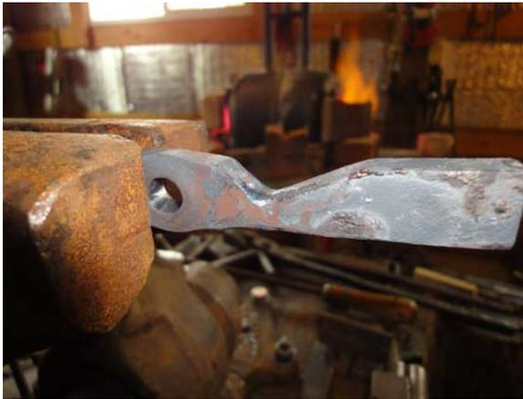
*Front notch with rounded edges*
